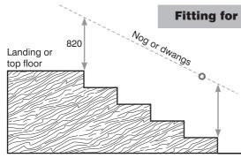
Fitting for handrail brackets on walls
