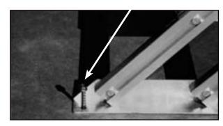
5. Fix handrail in correct position and securely fasten to the Stair Unit. Ensure bolts are tightened.
